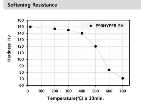
Vickers hardness after heat treatment (30minute).
