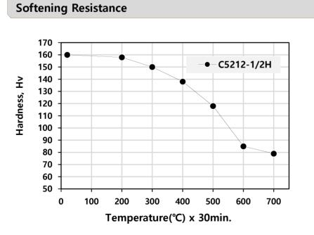
Vickers hardness after heat treatment (30minute). The diagram shows typical values.
